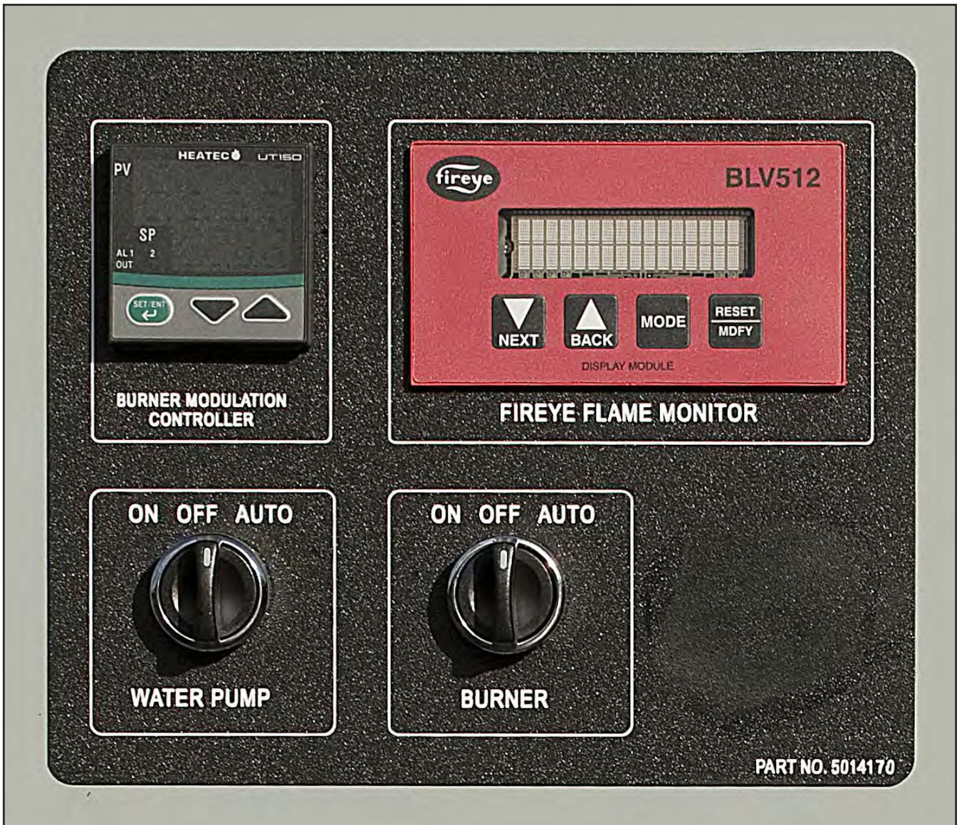
**Note:** Earlier panel marking FIREYE FLAME MONITOR is now BURNER DISPLAY
