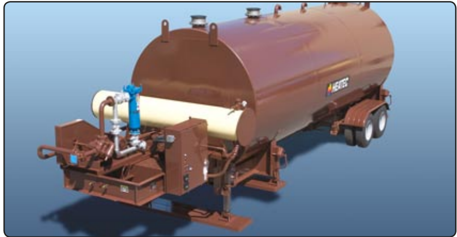
Portable 15,000 gallon fuel tank with double walls. Has 90 kw electric preheater (external).
