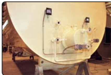
Horizontal fuel tank, built-in fuel preheater.
