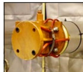
Loading and unloading valves are heated by heating cables.
