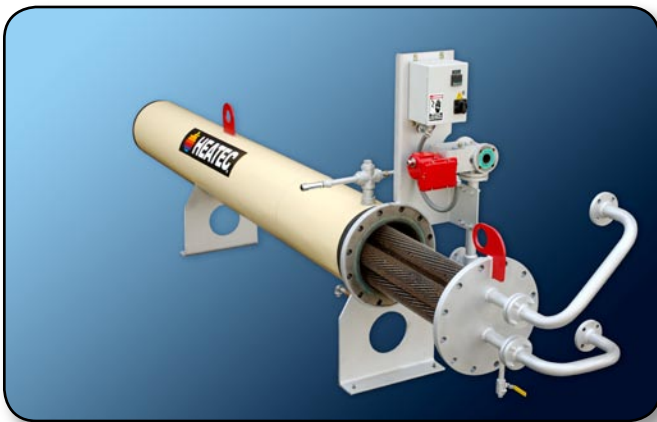
The entire coil bundle can be removed from the shell for cleanout of sludge and debris left by heavy fuel. A drain valve facilitates draining water that may accumulate in the shell.
