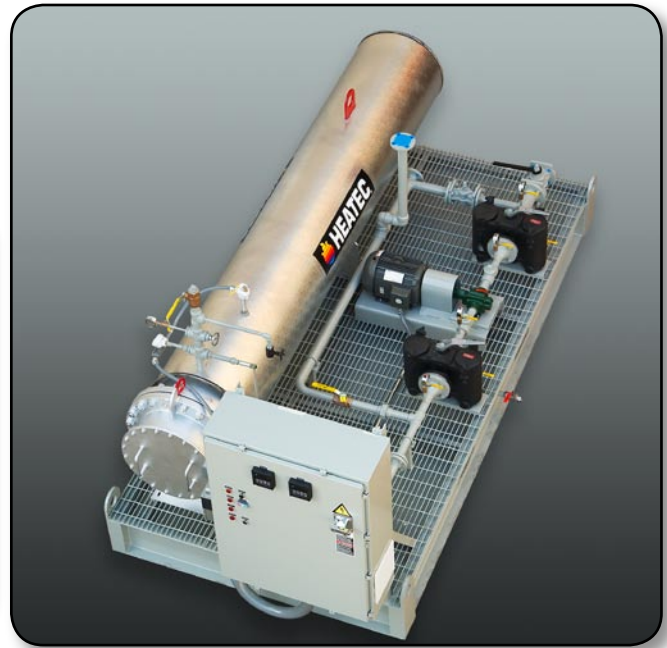
This is a 150 kW electric fuel preheater with a 100 degree temperature rise at 1,320 gph.
