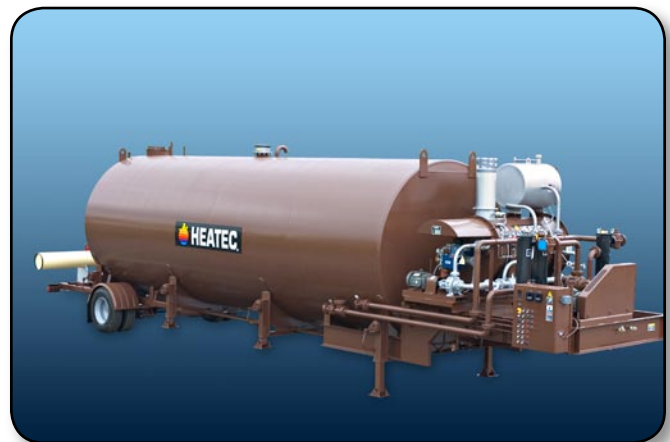
A portable fuel tank with a capacity of 20,000 gallons. A hot oil heater mounted on the gooseneck provides all the heat for the fuel preheater, which is mounted on a chassis extension. A fuel unloading pump and 3 sock filters are also mounted on the gooseneck. Retractable foundations facilitate fast setup.
