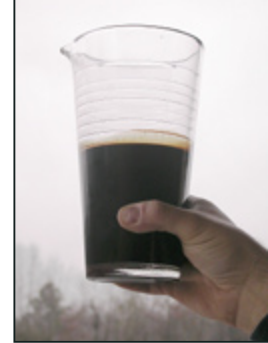
Old thermal fluid with bad signs.
