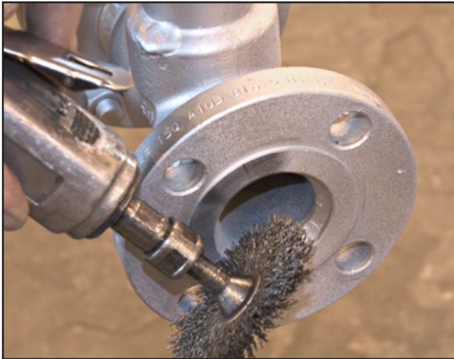
Figure 3. Cleaning surface that mates with gasket.
